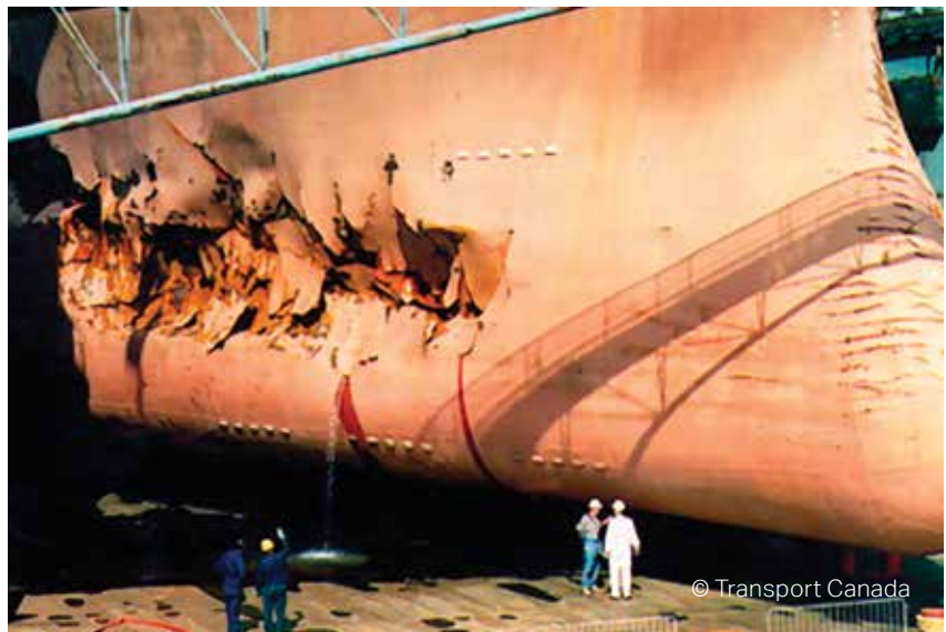
Damage from iceberg impact
