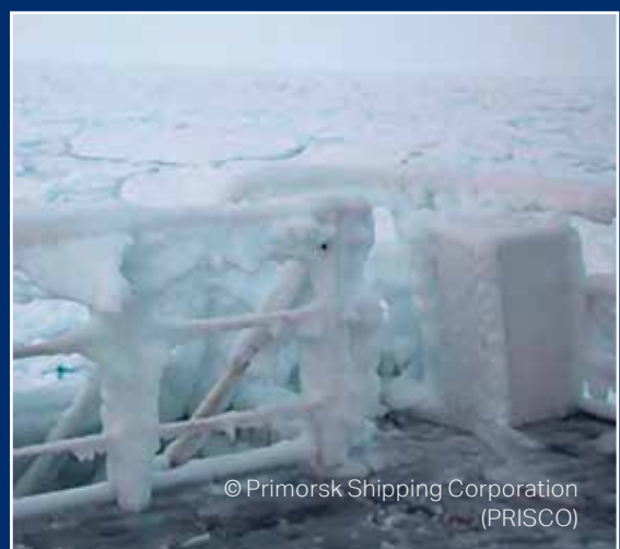
Ice accretion of stairway
